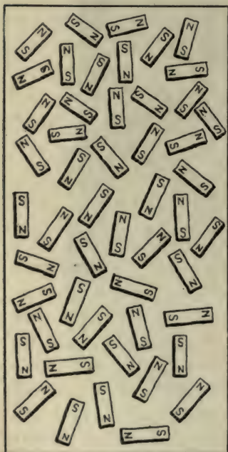
FIG. 107. Diagram of molecules in unmagnetized iron. The north and south poles of the molecules are supposed to be pointing in all directions.
